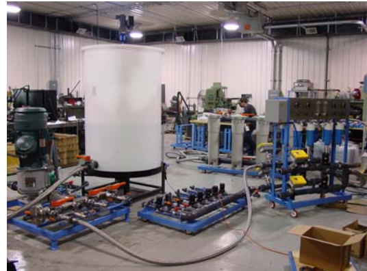
Laboratory Test System Developed To Test Commercial Filtration Units
