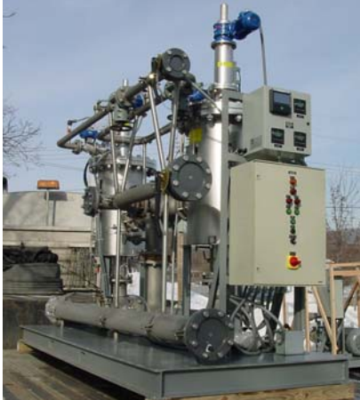
Pump and Filtration Package
