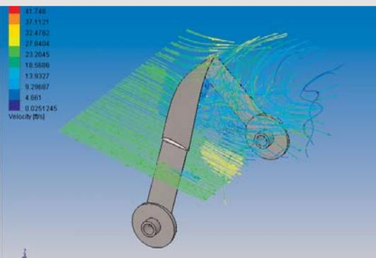
A feature in the latest COSMOSFloWorks includes a rotating frame of reference to simulate blade rotation. Results include forces generated by flow on the blades, and rotor torque. Analysis predictions closely matched experimental results.
