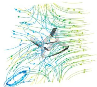
The water turbine uses helically shaped blades rotating at twice the velocity of the flow, and spinning the same direction regardless of flow direction. The turbine captures 35% of the water's energy, compared to 20% for conventional turbines. Anticipated costs for an open-river hydropower system should be \$400 to \$600/kW, lower than other systems. GCK Technology, San Antonio, is further developing the turbine.
