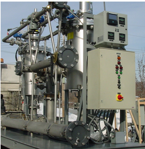
Pump and Filtration Package Design - Build: 100 HP, 500 GPM @ 225 PSI
