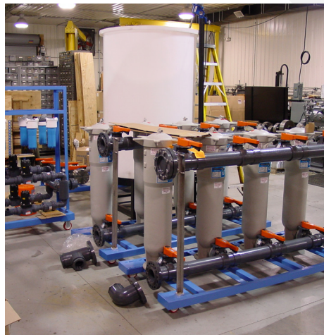
Laboratory Test System Developed To Test Commercial Filtration Units
