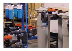
injection system, contaminate mixing tank, seawater supply pump, filtrate headers with baseline filters for comparison, backwash/underflow headers, backwash/ underflow cleanup filters, all piping, sample lines, valves, hoses, couplings, filtration component foundations, flow meters, and thermometers.
