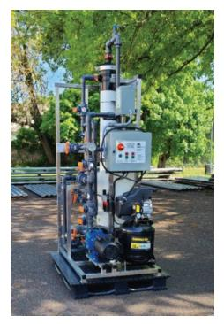
Used as an optimization and test system, Sigma Design Company's Model 4588 Pilot Ultrafiltration (UF) System for Brackish and Seawater is a fully operational, engineered membrane system used to determine the effectiveness and sizing of full scale UF equipment projects
