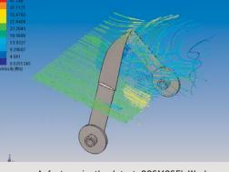
A feature in the latest COSMOSFloWorks includes a rotating frame of reference to simulate blade rotation. Results include forces generated by flow on the blades, and rotor torque. Analysis predictions closely matched experimental results.
