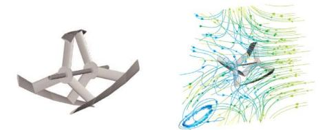
The water turbine uses helically shaped blades rotating at twice the velocity of the flow, and spinning the same direction regardless of flow direction. The turbine captures 35% of the water's energy, compared to 20% for conventional turbines. Anticipated costs for an open-river hydropower system should be \$400 to \$600/kW, lower than other systems. GCK Technology, San Antonio, is further developing the turbine.
