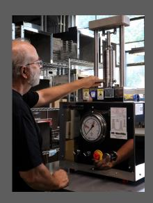
SIGMA DESIGN developed a high pressure testing chamber used to burst cell walls. The GM French Press uses a hydraulic press and carefully machined parts to produce pressures up to 40,000 psi. It opens new areas for development in medicine, cell research, tissue growth for replacements, large scale biomedical production by perfusion, and others. The medical device equipment complies with GLP, GCP, GTP and GMP standards.
